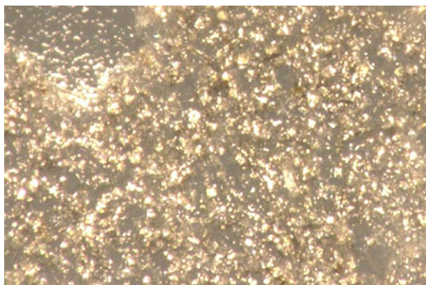
Figure 2. The micrograph of GFR-PA66 surface after cold spayed. [Color figure can be viewed in the online issue, which is available at wileyonlinelibrary.com.]
